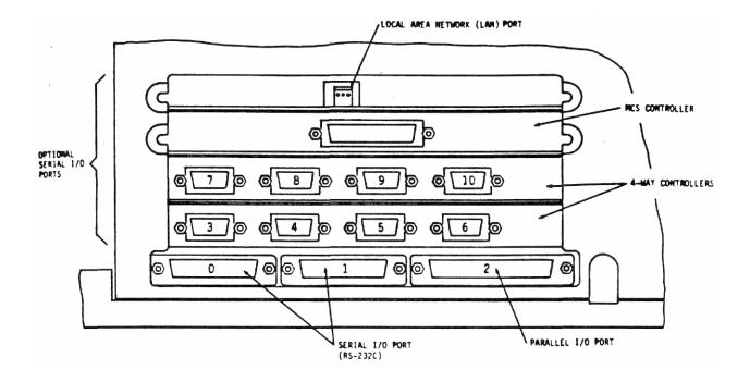
Figure 9-1. Rear View of Base Unit, Showing Location of All Ports
